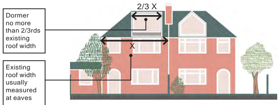
Figure 4.21a: Dormers on a semi-detached or detached house, no more than two thirds the width of the existing roof, and set in from the edge of a hipped roof (or a gable end).
