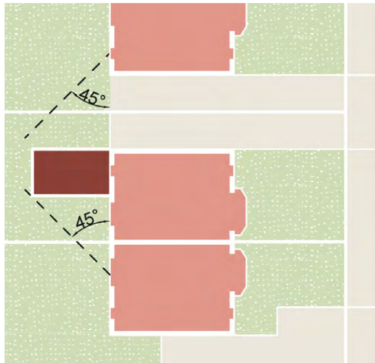
Figure 4.11b: An extension to a semi-detached house that is set away from neighbouring boundary, allowing for a deeper extension, up to a maximum of 45° as measured from the centre of the window of the nearest habitable room in the neighbouring properties.
